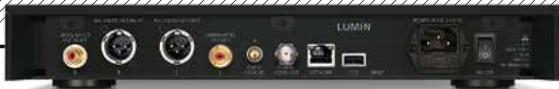
ABOVE: Simplicity itself as the diminutive T3 offers a USB-A port and wired Ethernet input (384kHz/32-bit; DSD512) alongside an S/PDIF output on BNC (192kHz/24-bit) and fixed/variable balanced/single-ended preamp outputs on XLRs/RCA's
